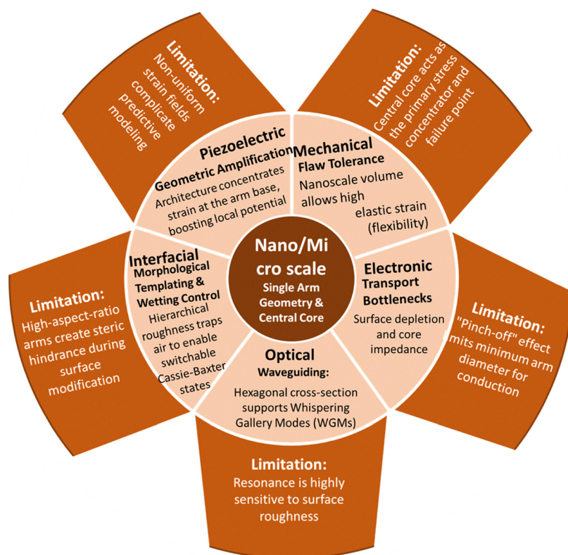
Fig. 45 Nano/micro scale geometric effects in T-ZnO. This figure details how the single-arm geometry and central core architecture influence properties such as flaw tolerance and optical waveguiding, while introducing bottlenecks like surface depletion and strain concentration at the arm base.
