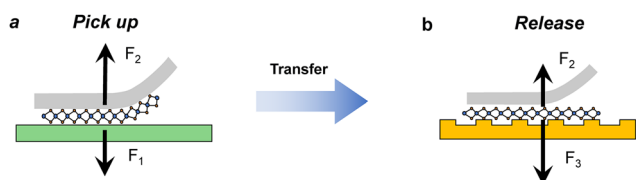
Fig. 4 The philosophy of 2D transfer. (a) The successful pick up requires F 2 > F 1 . (b) The successful release process requires F 3 > F 2 .
