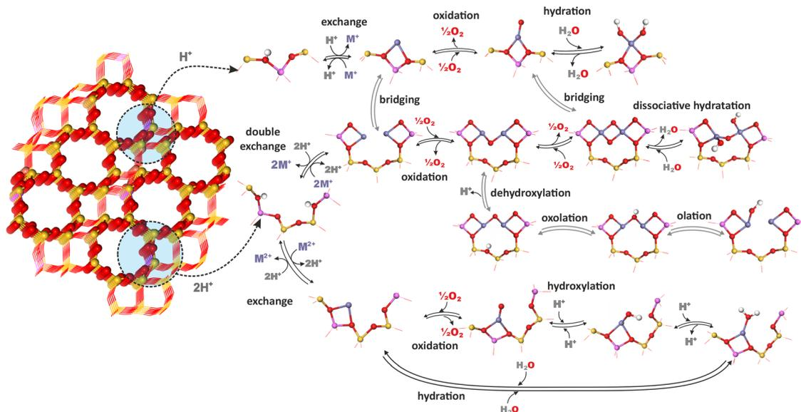
Fig. 13 Typical transformations of metal-containing zeolite centers controlled by thermodynamic conditions (temperature and  $O_2/H_2O$  pressures) associated with single ( $z_1$ ) and double ( $z_2$ ) exchange sites (tetrahedral  $AlO_4^-$  units). Atom color coding: O – red; Si – yellow; Al – pink; H – light grey; TMI ( $M^{n+}$ ) – pale blue.
