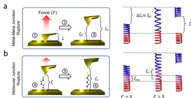
**Fig. 8** Atomic force microscopy-break junction. The schematic demonstration of the rupture of (a) a metal–metal junction and (b) a molecular junction. Panel is reprinted with the permission from ref. 109, Copyright (2023) Springer Nature.
