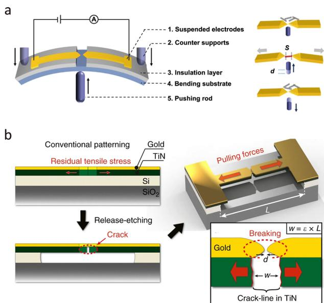
**Fig. 9** (a) Schematic illustration of MCBJ experimental setup and single molecule detection procedure. (b) Schematic demonstration of the nanogap fabrication through crack-defined break junction. Panel (a) is reprinted with permission from ref. 2, Copyright (2022) by Yi Zhao, under Creative Commons Attribution 3.0 license. Panel (b) is reprinted with permission from ref. 122, Copyright (2018), Springer Nature.
