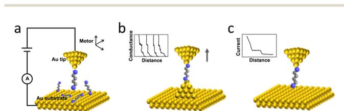
**Fig. 7** (a) The schematic illustration of the typical STM-BJ experimental setup. The single-molecule conductance can be measured via (b) hard-contact mode and (c) current-distance mode. Panel is reprinted with permission from ref. 2, Copyright (2022) by Yi Zhao, under Creative Commons Attribution 3.0 license.
