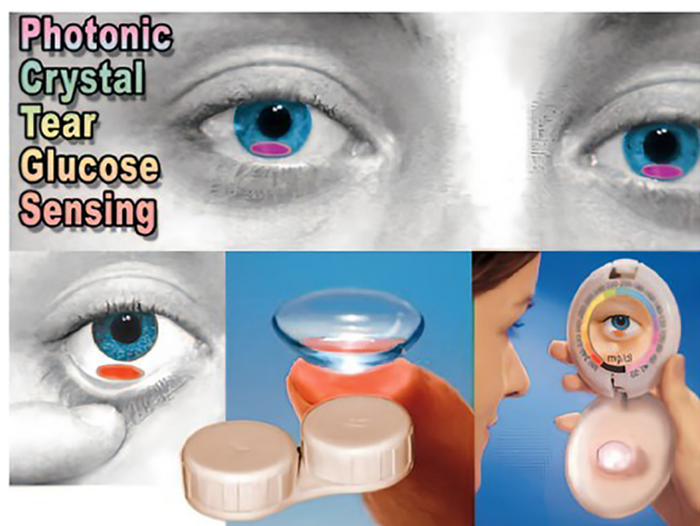
Fig. 79 Pictorial representation of boronic acid-based contact lens sensors for glucose concentration determination in tear fluid. Adapted with permission from ref. 182. Copyright (2004) The American Association for Clinical Chemistry.
