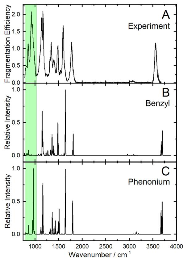
**Fig. 5** (A) The experimental IRIS spectrum of  $[\text{Tyr} - \text{NH}_3 + \text{H}]^+$  as monitored *via* the fragmentation channels given in Table 1. The calculated harmonic vibronic spectra for (B) the global minimum benzyl product and (C) the lowest energy phenonium product. Calculations were conducted at the  $\omega\text{B97X-D3BJ}/\text{def2-TZVPP}$  level of theory and a scaling factor of 0.97 was applied.<sup>91</sup>
