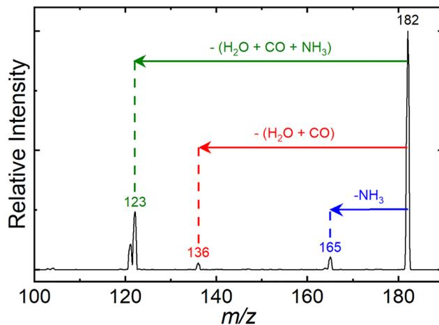
Fig. 2 The mass spectrum of  $[\text{Tyr} + \text{H}]^+$  following selection of  $m/z$  182 by Q1 and trapping in Q3. The  $m/z$  165,  $m/z$  136, and  $m/z$  123 products are formed *via* in-trap CID in Q3 following collision with background gas molecules.
