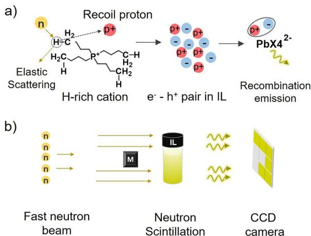
Fig. 6 (a) Illustration of the neutron scintillation by IL via generation of recoil proton after fast neutron bombardment, followed by recombination emission through the formation of electron–hole pairs. (b) Illustration of the neutron scintillation imaging using NIL as a scintillator. Fig. 6a and b adapted from ref. 99 with CC-BY-NC-ND 4.0 open access license from [American Chemical Society] [Kovalenko *et al.*, ACS Photonics, 2021, 8, 3357–3364], copyright 2021.
