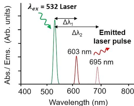
Fig. 9 Illustration of the spectral changes during photon downconversion of the 532 nm laser pulse due to stimulated Raman scattering in an IL;  $[C_2\text{mim}][\text{dca}]$  with Raman active dicyanamide anion. Adapted from ref. 105 with permission from [American Physical Society] [Palmer *et al.*, *Phys. Rev. Appl.*, 2023, **19**, 014052], copyright 2023.
