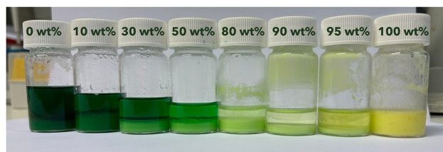
Fig. 4 Samples saturated with \text{Ni}(\text{CH}_3\text{SO}_3)_2 at 70 °C with varying initial MSA concentration from 0 wt% MSA (left) to 100 wt% MSA (right).
