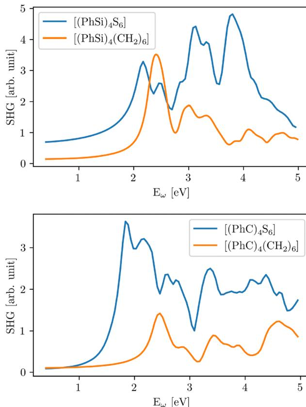
Fig. 20 Calculated SHG response of adamantane-type clusters  $[(\text{PhC})_4\text{S}_6]$  and  $[(\text{PhSi})_4\text{S}_6]$  with their S-free counterparts  $[(\text{PhC})_4(\text{CH}_2)_6]$  and  $[(\text{PhSi})_4(\text{CH}_2)_6]$ .
