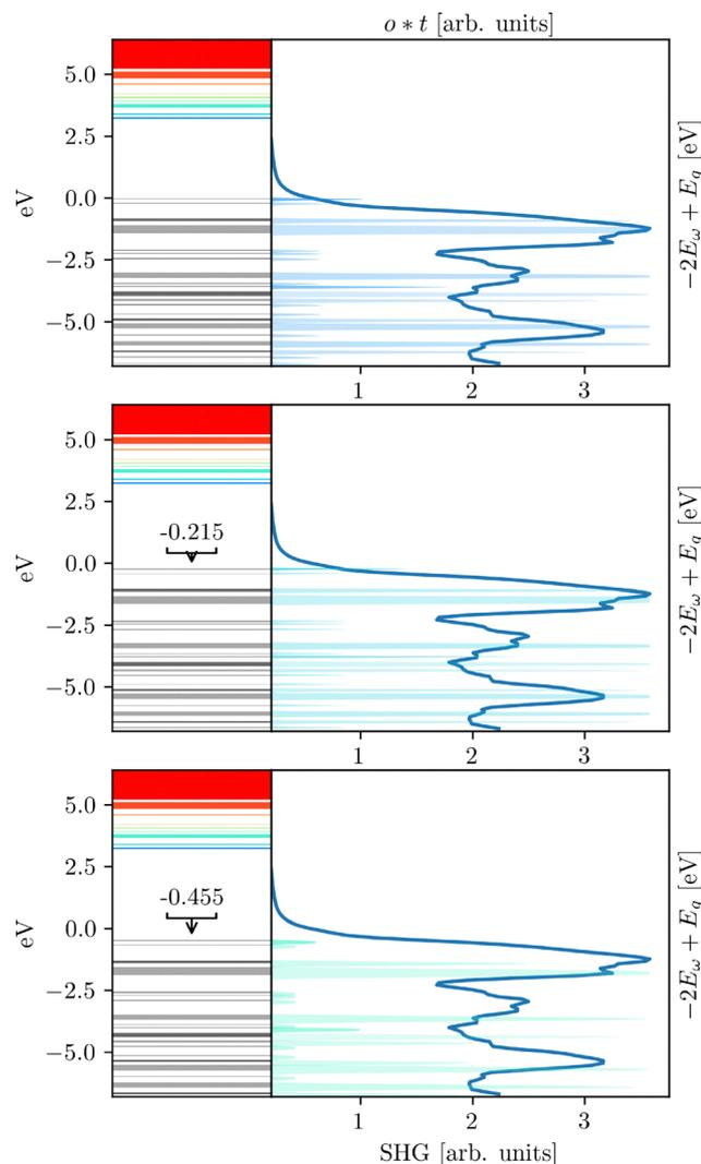
Fig. 10 Orbital group energy values of  $[(\text{PhSi})(\text{PhC})_3\text{S}_6]$  with corresponding scaled and shifted SHG response. The energy values of the origin orbital groups are shifted for a direct transition to the respective target orbital group  $t = 0$ ,  $t = 1$ , and  $t = 2$ .
