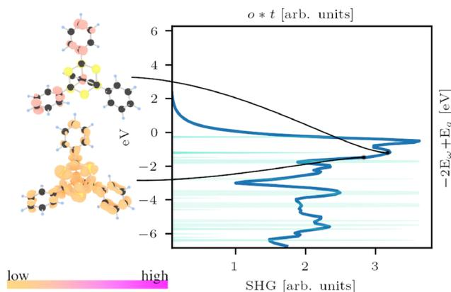
Fig. 17 Overlaps  $\rho$  of  $o = 1, 2$  with  $t = 2$ , related to the second peak of the SHG spectrum for  $[(\text{PhC})_4\text{S}_6]$ . The atoms are color-coded by atom type: S atoms are yellow, C atoms are black, and H atoms are light blue.
