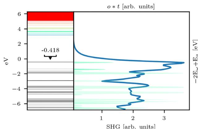
Fig. 13 Orbital group energy values of  $[(\text{PhC})_4\text{S}_6]$  with corresponding scaled and shifted SHG response. The energy values of the origin (occupied) orbital groups are shifted for a direct transition to the respective target (unoccupied) orbital group 3.
