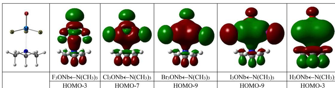
Fig. 2 Representations of X<sub>3</sub>ONb ← N(CH<sub>3</sub>)<sub>3</sub> molecular orbitals that are bonding between the NbOX<sub>3</sub> and N(CH<sub>3</sub>)<sub>3</sub> fragments. The position of each orbital relative to the highest occupied molecular orbital (HOMO) for the complex is indicated. All of the MO pictures share the same orientation. That common orientation is depicted on the left.
