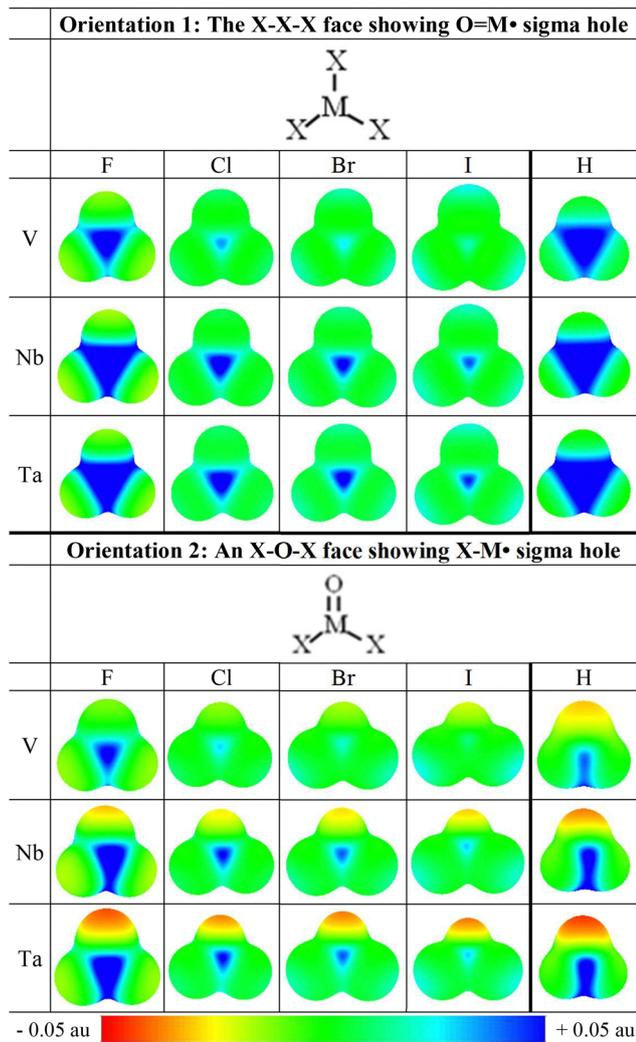
Fig. 1 ESP maps of the group 5  $\text{MOX}_3$  molecules. Two orientations are shown for each molecule, exposing the  $\text{O}=\text{M}\bullet$  sigma hole at the center of the  $\text{X}-\text{X}-\text{X}$  face (top), and a  $\text{X}-\text{M}\bullet$  sigma hole on a  $\text{X}-\text{O}-\text{X}$  face (bottom) of the molecule.
