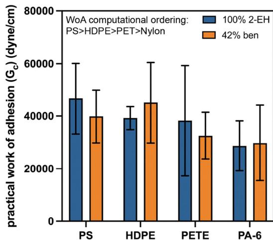
Fig. 6 Experimental Probe-tack comparison for select polyacrylate adhesives. Experiments were performed under aqueous conditions.
