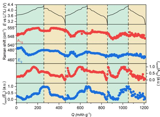
Fig. 3 Potential profiles of  $\text{LiNiO}_2$  *vs.*  $\text{Li}^+/\text{Li}$  (top), the fitted band positions (middle), and intensities (bottom) extracted from the *operando* Raman spectra and processed by PRISMA. Band intensities were normalised individually per cycle between 0 and 1.
