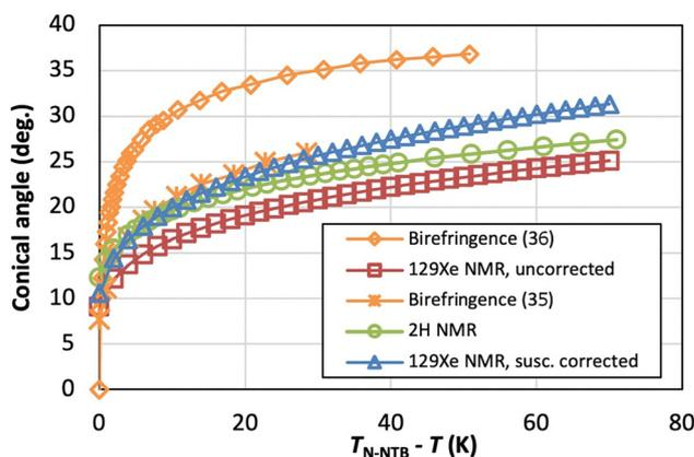
Fig. 5 Conical angle in CB7CB- $\text{D}_4$  as a function of temperature before (red squares) and after (blue triangles) bulk susceptibility correction to  $^{129}\text{Xe}$  shielding, and the conical angle derived from the  $^2\text{H}$  quadrupole splittings (cyan triangles). For comparison, also two results derived from birefringence measurements are shown (ref. 35 and 36).
