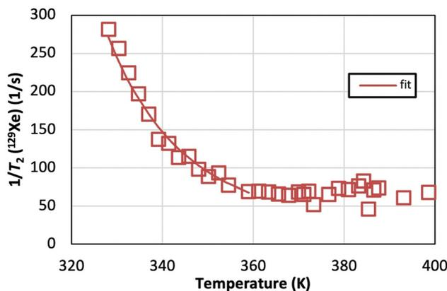
Fig. 9  $1/T_2$  ( $^{129}\text{Xe}$ ) as a function of temperature. The solid line is from eqn (15).
