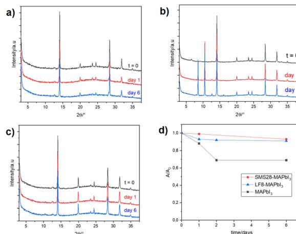
**Fig. 7** Humidity resistance test (RH75%) of a)  $\text{MAPbI}_3$ , b) **LF8**-I/ $\text{MAPbI}_3$ , c) **SMS28**-I/ $\text{MAPbI}_3$  thin films and d) degradation kinetics of the  $\text{MAPbI}_3$  layer over time.
