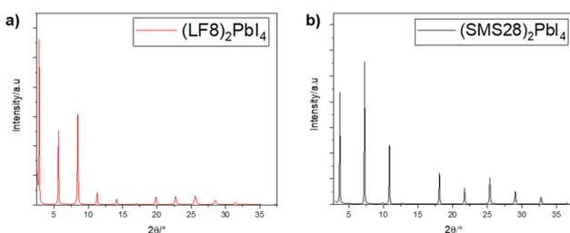
Fig. 2 XRPD patterns of a) (LF8)<sub>2</sub>PbI<sub>4</sub> and b) (SMS28)<sub>2</sub>PbI<sub>4</sub> thin films obtained by spin coating a solution of PbI<sub>2</sub> and RNH<sub>3</sub>I in DMSO.
