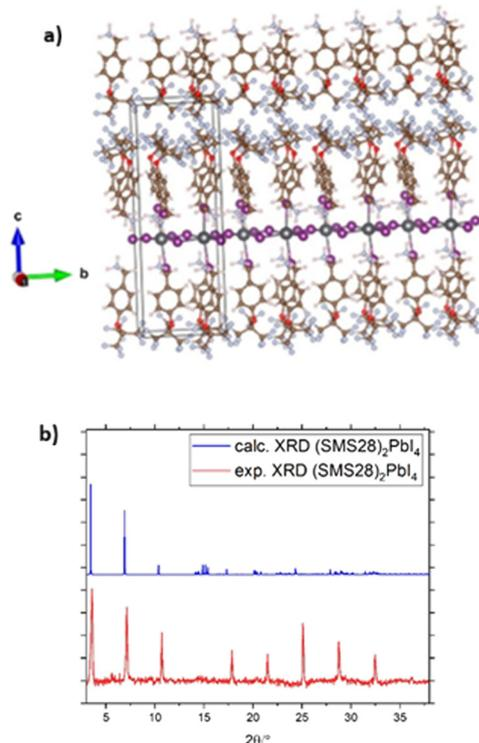
Fig. 4 a) Theoretical crystalline structure obtained from DFT geometrical optimization of  $(\text{SMS28})_2\text{PbI}_4$ , view along the “a” axis; b) DFT simulated and experimental XRPD patterns of  $(\text{SMS28})_2\text{PbI}_4$  crystal powders.
