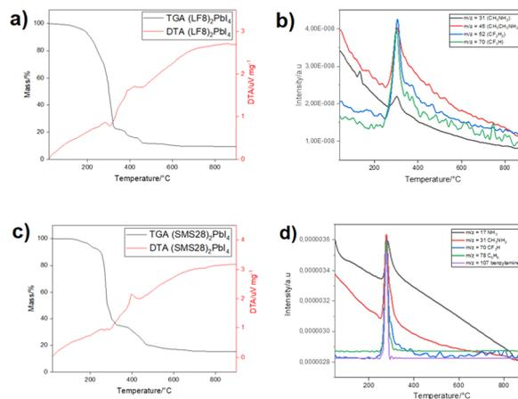
Fig. 3 a) TGA (black line) and DTA (red line) of (LF8)<sub>2</sub>PbI<sub>4</sub> powder; b) MS analysis coupled with DTA for (LF8)<sub>2</sub>PbI<sub>4</sub> powder; c) TGA (black line) and DTA (red line) of (SMS28)<sub>2</sub>PbI<sub>4</sub> powder; d) and b) MS analysis coupled with DTA for (SMS28)<sub>2</sub>PbI<sub>4</sub> powder.
