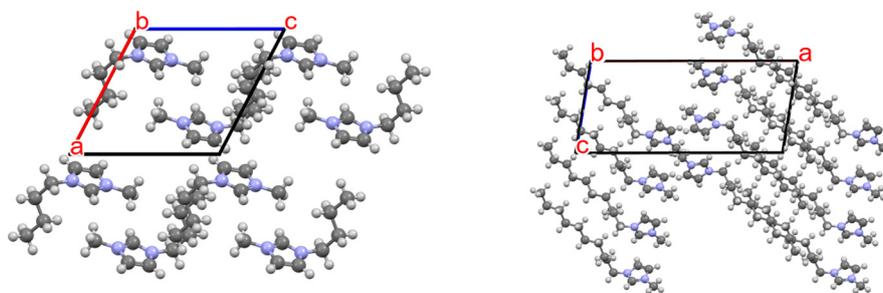
**Fig. 10** Packing diagrams of  $[\text{C}_4\text{mim}]$  cations (from  $[\text{C}_4\text{mim}][\text{PF}_6]$ , left)<sup>106</sup> vs.  $[\text{C}_{10}\text{mim}]$  cations (from  $[\text{C}_{10}\text{mim}][\text{PF}_6]$ , right).<sup>42</sup> The influence of the alkyl chains on the formation of the crystalline solid is seen with the interdigitation in the  $[\text{C}_{10}\text{mim}]$  packing diagram. Anions are omitted for clarity.
