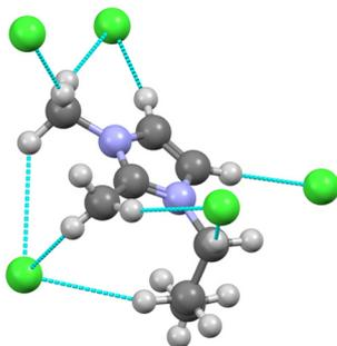
Fig. 5 The cation of the crystal structure of [C<sub>3</sub>Dime][Cl]<sup>51</sup> shown surrounded by multiple interacting chloride anions. Interactions between the cation hydrogens and the chloride anions are shown as the dashed blue lines.
