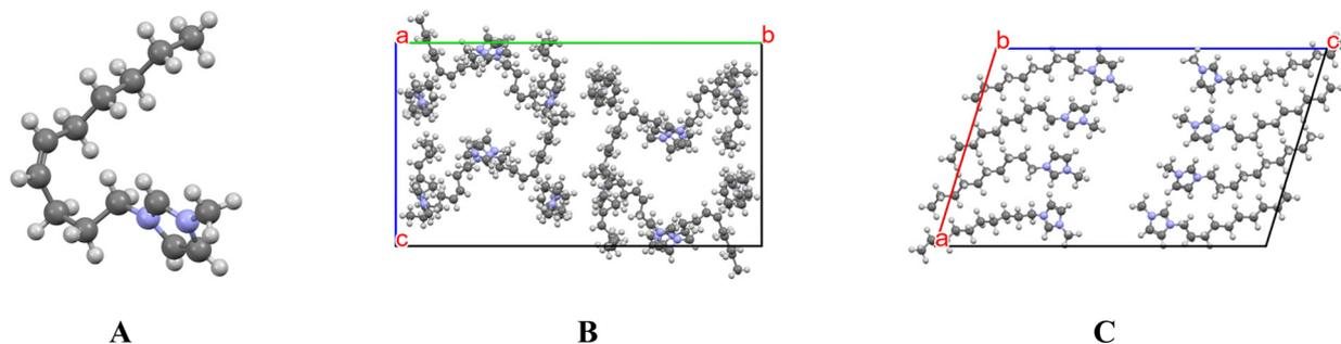
Fig. 14 (A) The cation of a dialkylated IL with a *cis*-alkene in the chain.<sup>104</sup> (B) Packing diagram of a *cis*-alkene bearing IL viewed down the crystallographic *a* axis contrasted with the fully saturated derivative (C) viewed down the *B* axis. Anions removed for clarity. The influences of the kinked alkyl chain is evident when contrasting the packing patterns of the two compounds. Disruption of alkyl interactions *via* chain kinking lowers melting points.
