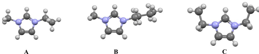
Fig. 8 A representation of the cations of [C<sub>2</sub>mim]<sup>90</sup> (A) and [C<sub>4</sub>mim]<sup>13</sup> (B). The [C<sub>2</sub>mim] cation is ‘more’ symmetric than the [C<sub>4</sub>mim], but both are considered less symmetric than the diethyl or [C<sub>2</sub>C<sub>2</sub>im] cation (C).<sup>91</sup>
