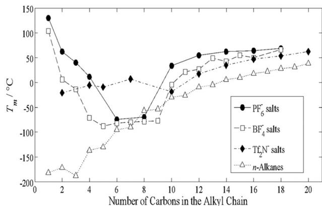
**Fig. 9** Melting point data for a dialkylated imidazolium ILs showing the influence of anion identity along with the discussed “alkyl-valley”. As alkyl chain length increases, a more predictable trend in melting points is observed. Reproduced from ref. 104 with permission from John Wiley and Sons, copyright 2010.
