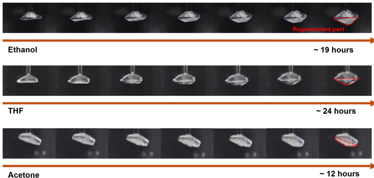
Fig. 8 Regeneration snapshots of paracetamol in top to bottom: ethanol, THF, and acetone.
