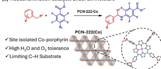
Figure 1. General overview of this work (a) Solution reactor dosing for high-throughput MOF catalyst assays used in this work and (b) general reaction scheme for the amination reaction in this communication, with a zoomed-out of the Porphyrin linker in PCN-222(Co).
