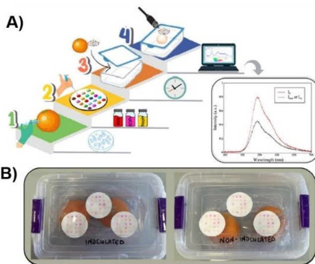
Fig. 9: A) workflow of sensing by the fluorescent array; B) Photos of the packaging used to detect orange storage and contamination. Reprinted with permission of Ref. 59. Copyright 2024. Royal Society of Chemistry.
