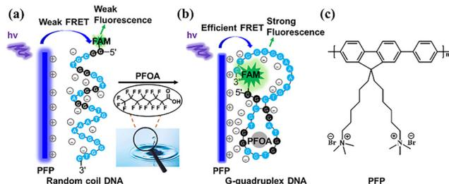
**Scheme 1** (a) and (b) Schematic illustration of a fluorescent conjugated polymer-based ratiometric aptasensor for sensitive detection of PFOA. (c) Chemical structure of the cationic polyfluorene (PFP).
