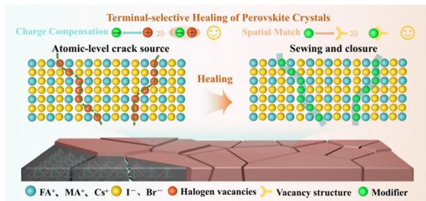
Fig. 1 Schematic diagram of the surface grain boundaries and atomic-level cracks on the crystal surface of perovskite films, and an illustration of the repair strategy.
