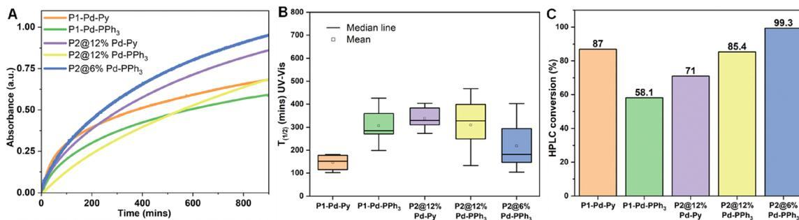
Fig. 2 (A) Kinetic profiles of encapsulated **P1** and covalently attached **P2** NPs in a pro-DNP (**4**) (100  $\mu$ M) to DNP (**5**) conversion monitored by UV-Vis over time at  $\lambda = 400$  nm in water at 37  $^{\circ}$ C using 30  $\mu$ M of Pd; (B) T<sub>1/2</sub> comparison of the **P1** and **P2** NPs in the formation of DNP (**5**); T<sub>1/2</sub> (time taken for 50% formation of DNP (**5**) by UV-Vis, mean of multiple runs); (C) HPLC conversion of DNP (**5**) after 24 h.
