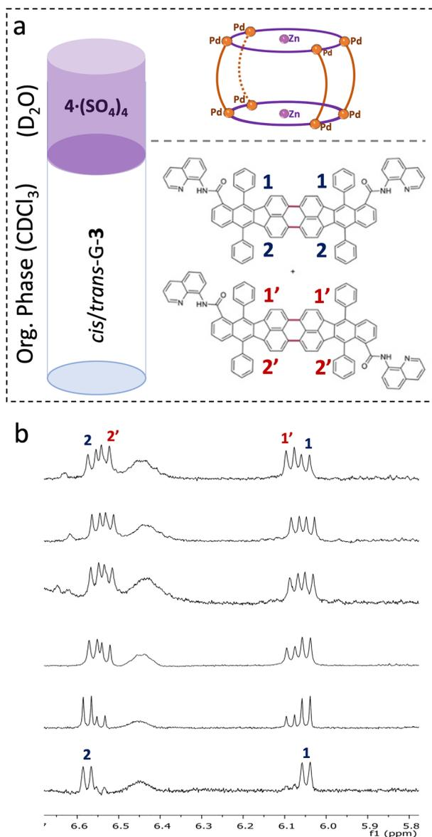
Fig. 2 (a) Schematic representation of the biphasic system designed to purify *cis/trans*-G-3 NGs. (b) Stacked partial  $^1\text{H}$  NMR spectra of *cis/trans*-G-3 isomeric mixture, showing spectral changes upon selective host-guest complexation of *trans*-G-3 along the time (15 min intervals; time = 0, top spectrum; time = 75 minutes, bottom spectrum).
