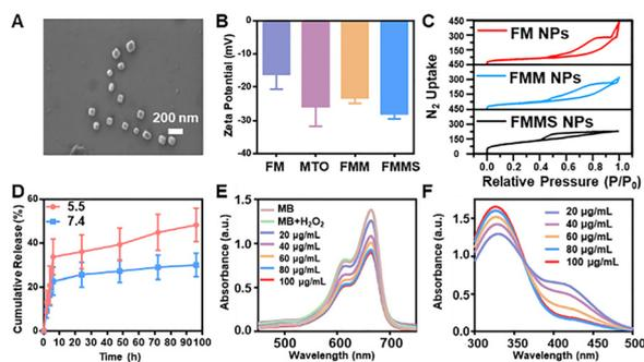
Fig. 2 (A) SEM image of FMMS NPs. (B) Zeta potentials of FM NPs, MTO, FMM NPs, and FMMS NPs ( $n = 3$ ). (C) Nitrogen absorption curves for FM NPs, FMM NPs, and FMMS NPs. (D) Cumulative releases of MTO from FMMS NPs under indicated pH conditions ( $n = 3$ ). (E) Absorbance spectra of MB with indicated concentrations of FMMS NPs. (F) GSH consumption and GSSG generation of FMMS NPs.
