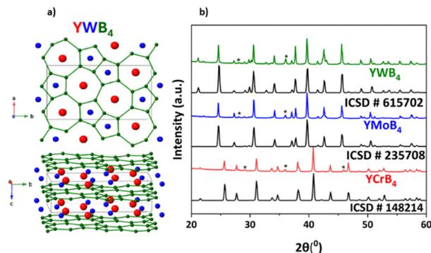
Fig. 1 (a) Crystal structure of YWB<sub>4</sub>, (b) powder X-ray diffraction patterns for YCrB<sub>4</sub>, YMoB<sub>4</sub>, and YWB<sub>4</sub>. Reference patterns: ICSD 148214,<sup>45</sup> 235708,<sup>46</sup> and 615702,<sup>43</sup> respectively. (\*) – peaks for YB<sub>4</sub>.
