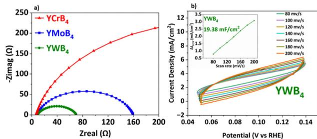
Fig. 3 (a) Electrochemical impedance spectroscopy (EIS) Nyquist plots of YCrB<sub>4</sub>, YMoB<sub>4</sub>, and YWB<sub>4</sub>. (b) Cyclic voltammety curve of YWB<sub>4</sub>. (Inset showing the difference in the current density of  $\Delta J (J_a - J_c)$  at 0.1 V vs. RHE plotted against the scan rate is fitted to a linear regression to estimate  $C_{dl}$ .)
