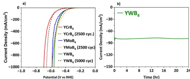
Fig. 4 (a) Polarization curve of YCrB<sub>4</sub>, YMoB<sub>4</sub>, and YWB<sub>4</sub> before and after 2500, 2500, and 5000 cycles, respectively. (b) Chronoamperometry curve of YWB<sub>4</sub> for 24 h.
