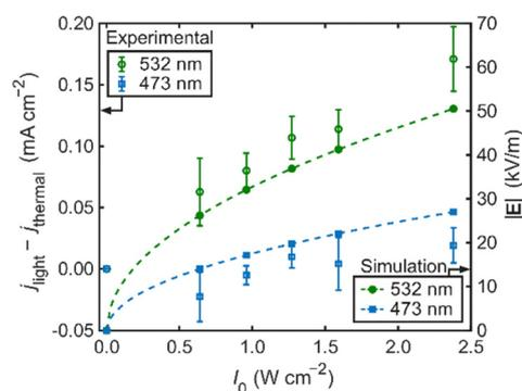
**Fig. 4** Difference between plasmon and thermal current densities (left y-axis) and simulated magnitude of the electric field at the surface of the nanoparticle (right y-axis) as a function of the incident light intensity at 473 and 532 nm.
