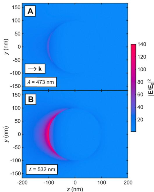
Fig. 1 Simulated electromagnetic field enhancement in the vicinity of a 200 nm Au nanosphere in water under excitation of  $2.38 \text{ W cm}^{-2}$  of (A) 473 and (B) 532 nm.
