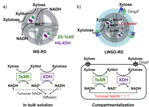
Fig. 1 Schematic illustrations of the enzyme cascade reaction in both a bulk solution and a compartmentalized environment. (a) In a bulk solution, the free diffusion of the intermediate xylitol and the cofactor NAD + results in a lower conversion efficiency of the cascade. (b) In a compartmentalized environment, the effective concentrations of enzymes and cofactors are significantly increased. This confinement serves to minimize the diffusion of cofactors into the external solution, thereby enhancing the reaction rate and the efficiency of cofactor recycling in enzymatic reactions.
