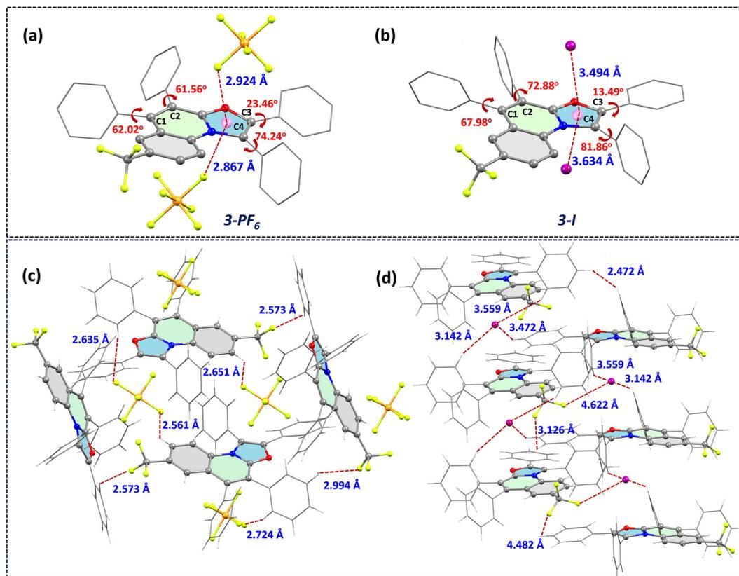
Fig. 4 (a) and (b) Crystal structure analysis and comparison of key parameters between **3-PF<sub>6</sub>** and **3-I**. (c) Non-covalent interactions between the fluorine atoms of the hexafluorophosphate anion and the hydrogen atoms of the phenyl rings of **3-PF<sub>6</sub>**. (d) Non-covalent interactions between the iodide anion and the hydrogen atoms of the phenyl rings of **3-I**.
