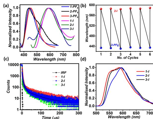
Fig. 3 (a) Solid-state photoluminescence (PL) spectra of **1-PF<sub>6</sub>**, **2-PF<sub>6</sub>**, **3-PF<sub>6</sub>**/**1-I**, **2-I**, and **3-I** pairs. (b) Reversible counter-anion exchange of **2-PF<sub>6</sub>**/**2-I** pairs up to 6 cycles. (c) Time-resolved PL decay of the iodide compounds in the solid state at room temperature. (d) The delayed PL spectra of the iodide compounds at 77 K.
