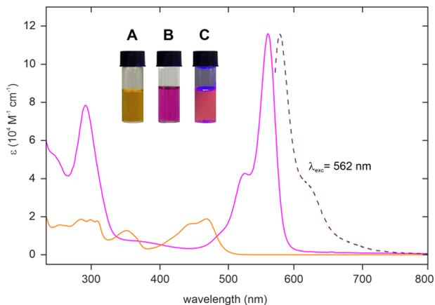
**Fig. 3** UV-vis absorption spectra of **3-Zn** (orange solid line) and **5-Zn** (violet solid line) in  $\text{CH}_3\text{OH}$  at 298 K. The dotted line shows the fluorescence spectrum of **5-Zn** in  $\text{CH}_3\text{OH}$  recorded upon excitation at 562 nm at 298 K. The inset shows the colour of methanolic solutions of (A) **3-Zn**, (B) **5-Zn**, and (C) **5-Zn** under UV light (365 nm).
