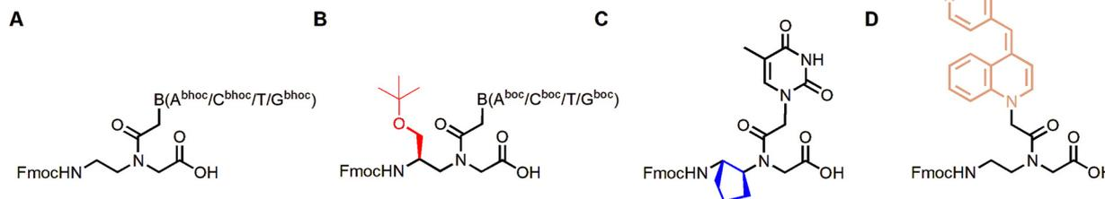
Fig. 1 Chemical structures of Fmoc-protected PNAs and the BisQ-FIT-PNA monomer: (A) unmodified, amino-ethyl-glycine (aeg)-PNA monomers ( $A^{bhoc}/C^{bhoc}/T/G^{bhoc}$ ), (B) gamma-modified,  $\gamma$ -(L)-serine PNA monomers ( $A^{boc}/C^{boc}/T/G^{boc}$ ), (C) cyclopentane, cpT monomer, and (D) BisQ monomer.
