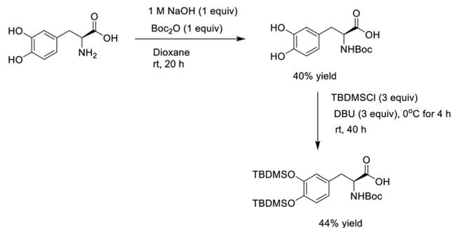
**Scheme 6** Reaction scheme for the protection of L-DOPA.
