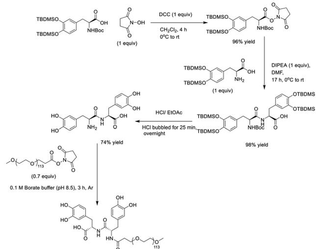
**Scheme 7** Reaction scheme of the synthesis of mPEG-(DOPA)<sub>2</sub>.
