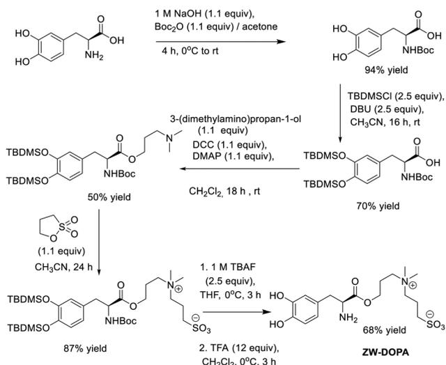
**Scheme 10** Synthesis of sulfobetaine DOPA zwitter ion.
