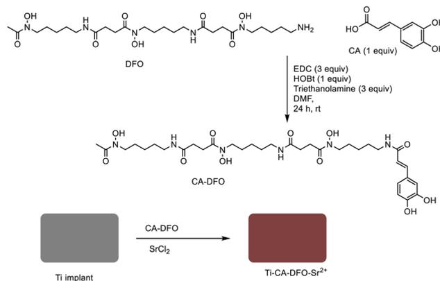
Scheme 23 Synthesis of caffeic acid–deferoxamine (CA-DFO) conjugate and polymerization with SrCl<sub>2</sub> on Ti.
