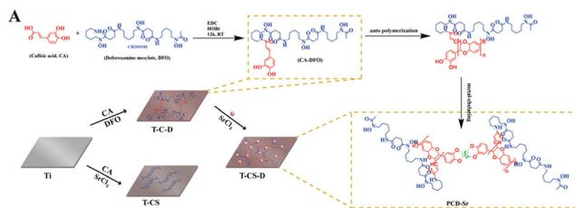
**Fig. 19** Schematic diagram of the chemical synthesis of Ti modified with CA-DFO and Sr<sup>2+</sup>(T-CS-D). Reproduced with permission from ref. 72. Copyright 2023 John Wiley and Son.
