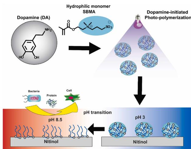
**Fig. 11** pSBMA/DA synthesized *via* dopamine-initiated photo-polymerization method and deposition on nitinol through pH-induced aggregation formation. Reproduced with permission from ref. 48. Copyright 2022 Elsevier.
