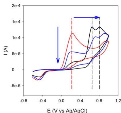
**Fig. 10** CV curves of dopamine at 3.5 mM in Tris buffer (red line), in Tris buffer containing 43.0 mM boric acid (blue line), and in Tris buffer containing 430 mM boric acid (black line). Reproduced with permission from ref. 40. Copyright 2017 American Chemical Society.
