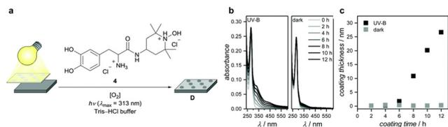
**Fig. 8** Light-induced polymer film formation on surfaces generating spatially confined antibiofilm domains. (a) Synthetic route for the photo-polymerization onto titanium substrates. (b) UV-vis spectroscopic monitoring of catechol oxidation and catecholamine polymerization. (c) Coating thickness of polymer films deposited on silicon substrates under UV irradiation. Reproduced with permission from ref. 29. Copyright 2019 Royal Society of Chemistry.
