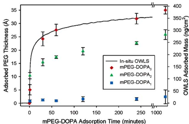
Fig. 5 Time-dependent adsorption of mPEG-DOPA onto TiO<sub>2</sub>. Reproduced with permission from ref. 27. Copyright 2005 American Chemical Society.
