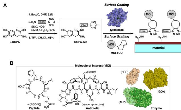
**Fig. 9** Overview of the bioorthogonal material surface functionalization *via* Tet-TCO ligation of molecules of interest (MOIs) through L-DOPA grafting. Reproduced with permission from ref. 33. Copyright 2019 American Chemical Society.
