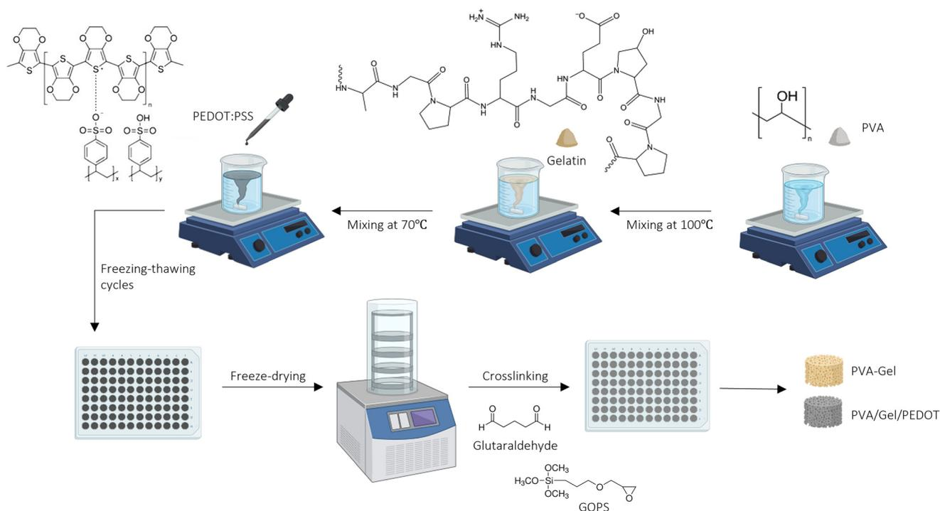
**Fig. 1** Schematic (created with BioRender) on the workflow of the scaffold fabrication. PEDOT:PSS is the acronym for poly(3,4-ethylene dioxythiophene):poly(styrene sulfonate), PVA is the acronym for poly(vinyl)-alcohol, and GOPS is the acronym for (3-glycidyloxypropyl) trimethoxysilane.
