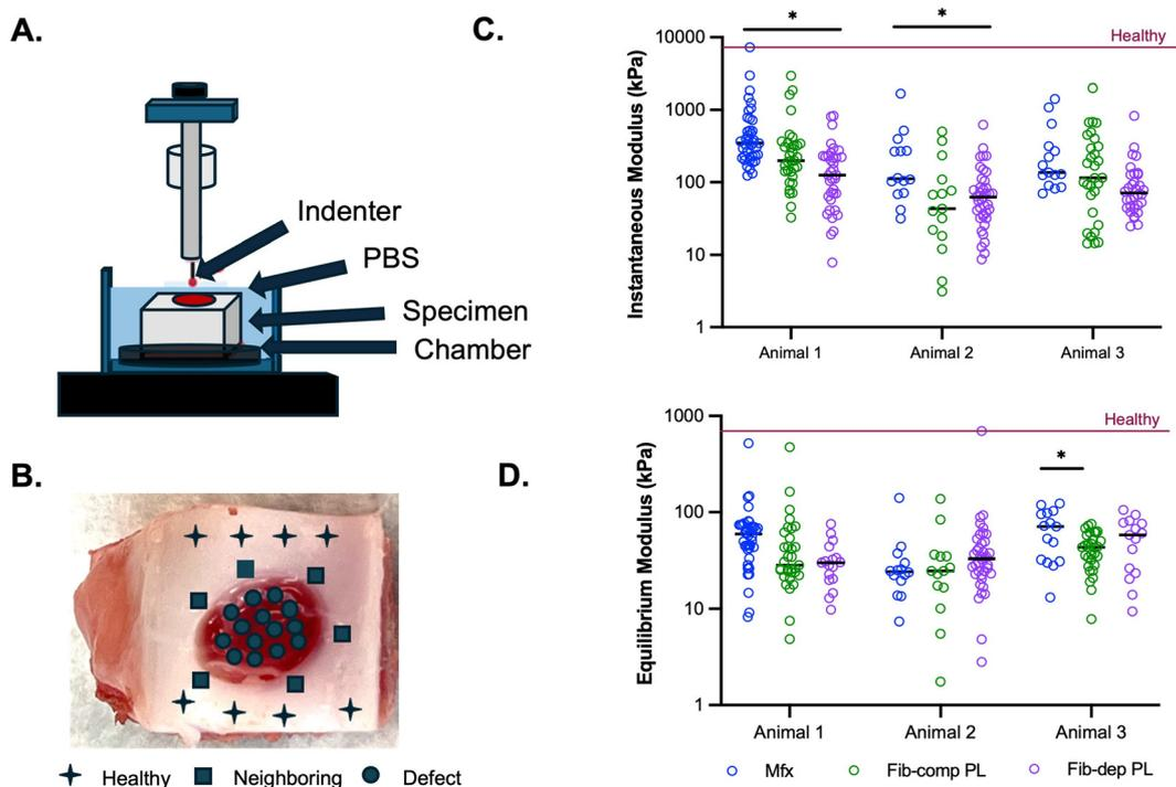
**Fig. 6** [A] Schematic of Biomomentum Mach-1 indentation testing. [B] Representative image of positions on cartilage defect that were tested. [C] Instantaneous modulus and [D] equilibrium modulus of each group, broken down by animal. Red line indicates healthy tissue. \* $p < 0.05$ .
