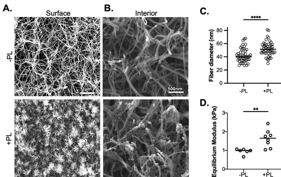
**Fig. 2** Scanning electron micrographs of fibrin gels without or with platelet lysate (PL) obtained [A] on the surface or [B] within gels. Scale bar = 2  $\mu$ m and 500 nm, respectively. [C] Quantification of fibrin fiber diameter within the interior of the gel. *n* > 40 fibers per group from 3 images. [D] Equilibrium modulus of fibrin gels without or with PL augmentation. *n* = 6–8 per group. \*\**p* < 0.01, \*\*\*\**p* < 0.0001.
