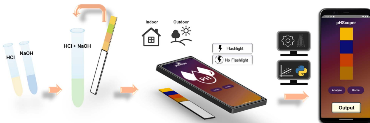
Fig. 1 The workflow for ML-based pH detection on a smartphone application.
