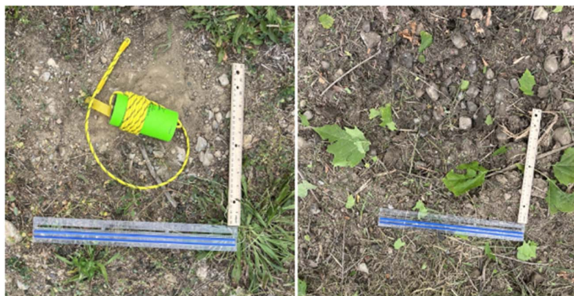
Fig. 2 Site 1 area measurement pre-blast (left) and post-blast (right) of cast booster.
