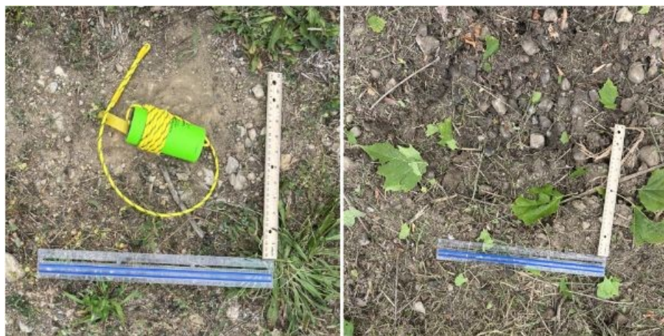
Figure 2. Site 1 area measurement pre-blast (left) and post-blast (right) of cast booster.
