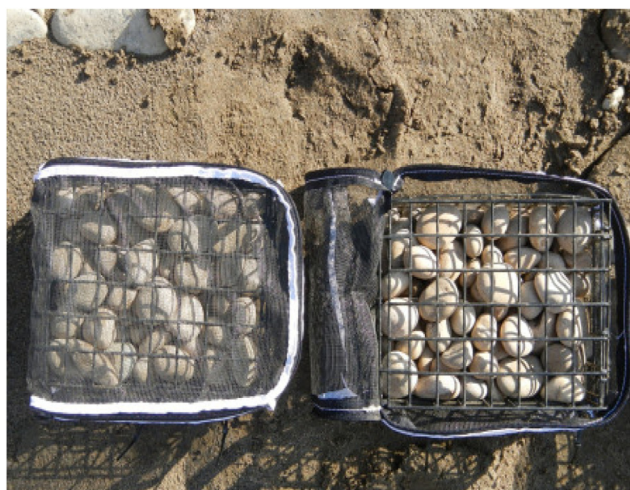
Fig. 4 Example of a field-deployable cage used in an environmental metabolomics study. Each cage is used to house two dragonfly nymphs ( Ophiogomphus colubrinus ). The photographs show the 1 mm mesh basket fully zipped for deployment (left) and open prior to closure (right). Reprinted from Applied Environmental Metabolomics, R. Brua, J. Culp, S. Pomfert, D. Halliwell, Chapter 19 – NMR-based metabolomics of dragonfly nymphs exposed to multiple stressors: An approach for field assessments to diagnose effects, Pages 273–289, Copyright (2022), with permission from Elsevier.
