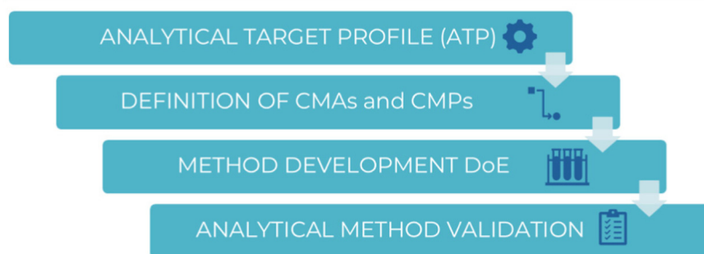
Fig. 2 Analytical quality by design workflow used for method development.
