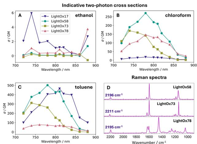
**Fig. 2** Indicative two-photon cross section of LightOx compounds in (A) ethanol, (B) chloroform and (C) toluene. (D) Raman spectra of LightOx compounds in the solid state with the peak wavenumber of the alkyne (C≡C) stretch labelled.
