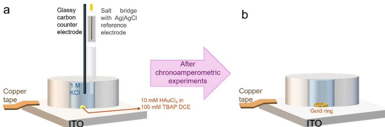
**Fig. 1** (a) Schematic for ring deposition with a droplet (yellow) of 10 mM  $\text{HAuCl}_4$  in 100 mM TBAP in DCE onto the ITO surface in the cell. A solution of 1 M KCl (blue) was used as the supporting electrolyte. Chronoamperometry was run from the potential  $-0.65$  V for 0.5 s to 0.3 V for 0.5 s and cycled twice. (b) Schematic for the cell setup displaying the deposited gold nanoring at the interface of the ITO, droplet and supporting electrolyte phase.
