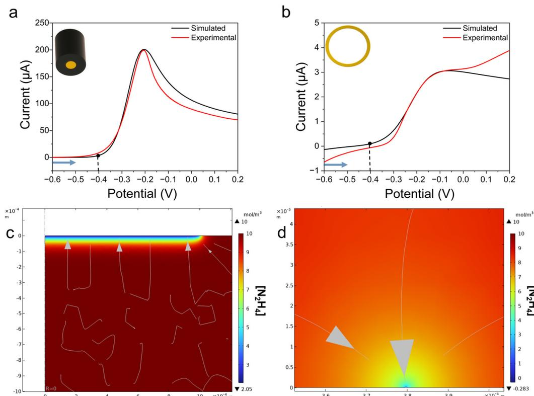
**Fig. 3** Overlaid cyclic voltammograms of simulated data (black trace) and experimental data (red trace) are shown in (a) and (b) for a gold macroelectrode and the gold single nanoring, respectively. (c) Shows a concentration profile for hydrazine oxidation on the gold macroelectrode at 8 s,  $-0.44$  V, (black dot) and (d) shows the concentration profile on the gold nanoring at 13.5 s,  $-0.43$  V. Blue directional arrows indicate scan direction.
