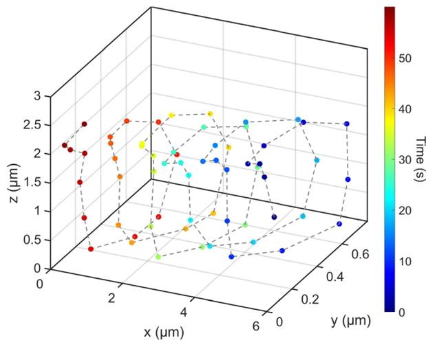
Fig. 7 Trajectory of the microrod swimming at  $0.56 \text{ V } \mu\text{m}^{-1}$  and  $90 \text{ mHz}$ , with positions colour-coded by time. This trajectory corresponds to Fig. 6, the swimming velocity is  $v_x = -0.08 \text{ } \mu\text{m s}^{-1}$ .
