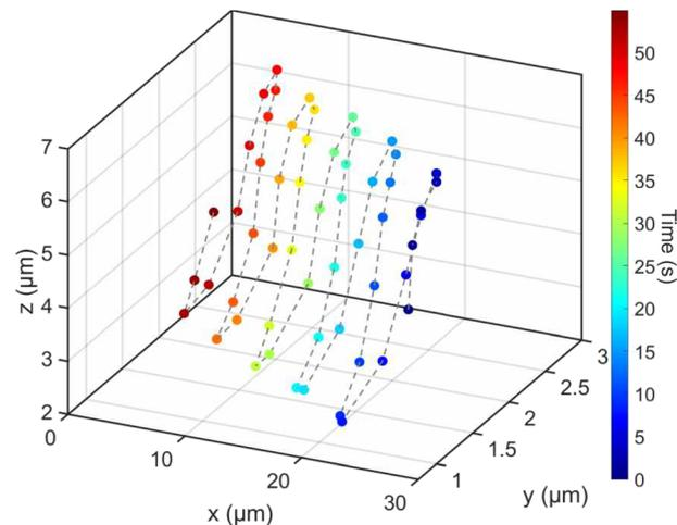
Fig. 9 3D trajectory of the microrod swimming at  $0.56 \text{ V } \mu\text{m}^{-1}$  and  $90 \text{ mHz}$ , with positions colour-coded by time. This trajectory corresponds to Fig. 8, the swimming velocity is  $v_x = -0.5 \text{ } \mu\text{m s}^{-1}$ .
