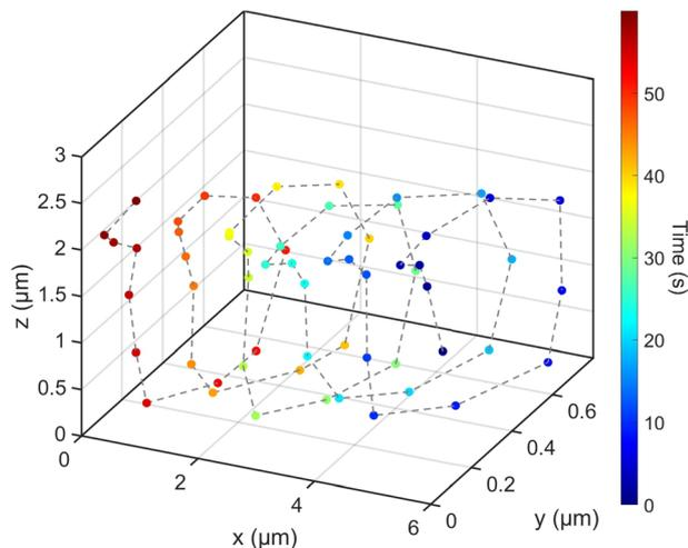
Fig. 7 Trajectory of the microrod swimming at  $0.56 \text{ V } \mu\text{m}^{-1}$  and  $90 \text{ mHz}$ , with positions colour-coded by time. This trajectory corresponds to Fig. 6, the swimming velocity is  $v_x = -0.08 \text{ } \mu\text{m s}^{-1}$ .
