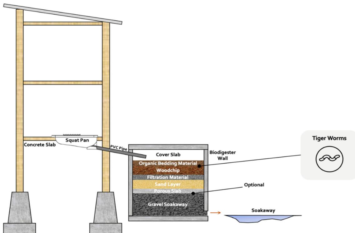
Fig. 1 Structural design of TWT, adapted from ref. 1.
