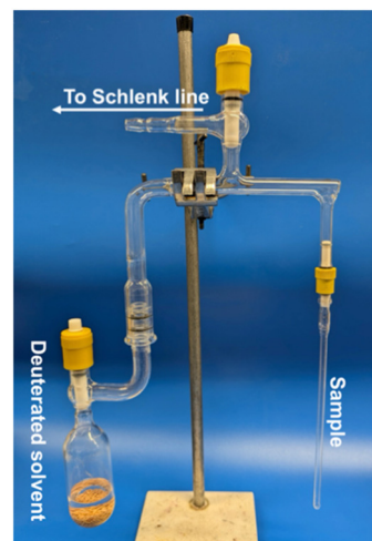
Fig. 13 Vacuum transfer apparatus for condensation of deuterated solvents onto crystalline solid-samples. The NMR tube containing the sample is placed inside a dewar containing a suitable cryogen.
