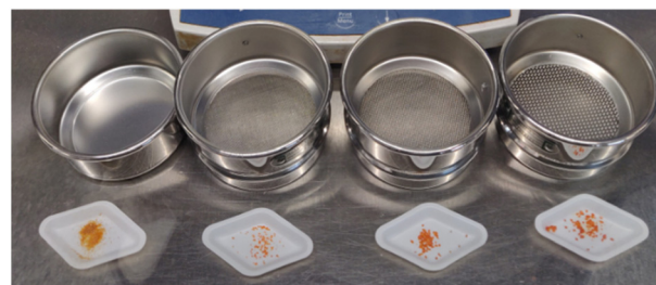
Fig. 4 Graded sieving of crystals (from left to right) 0.25, 0.5 and 1 mm sieves.
