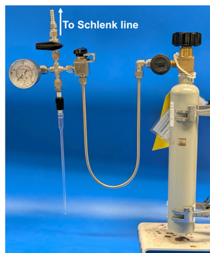
Fig. 7 Custom built drying tube packed with Pd/C and 3 Å molecular sieves for removing impurities from \text{CD}_4 .
