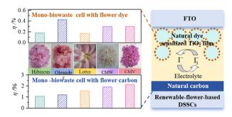
Renewable flower-based dye-sensitized solar cells using natural dye and natural carbon counter electrode
