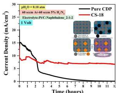
**SnO<sub>2</sub> modified CsH<sub>2</sub>PO<sub>4</sub> (CDP) protonic electrolyte for an electrochemical hydrogen pump**
