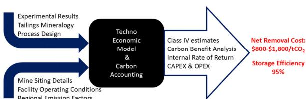
**Techno-economic analysis of indirect carbonation processes for carbon sequestration using mining waste**
