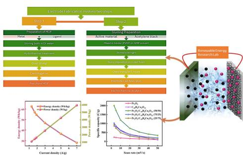
**Evaluating the potential of Pr<sub>2</sub>O<sub>3</sub>/C<sub>18</sub>H<sub>6</sub>Cu<sub>3</sub>O<sub>12</sub> composites as positrodes with sustainable energy-power density for battery-supercapacitor hybrids**
