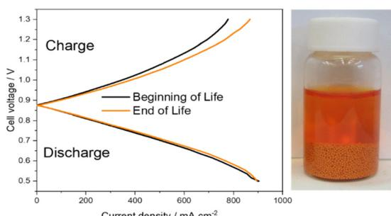
**Solid bromine complexing agents: long-term solution for corrosive conditions in redox-flow battery**
