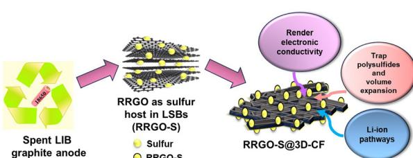
**Reduced graphene oxide derived from the spent graphite anodes as a sulfur host in lithium–sulfur batteries**
