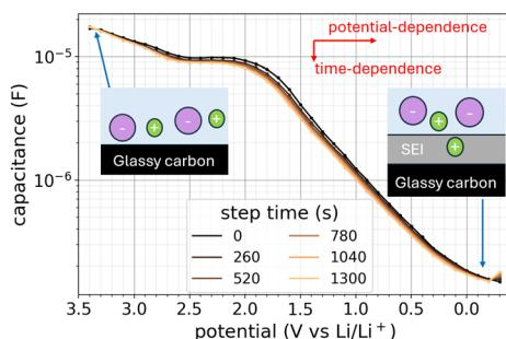
**Double layer capacitance as a sensitive metric to monitor the formation of solid electrolyte interphases in Li-ion batteries**
