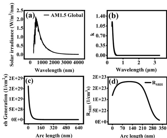
Fig. 1 Optical and electrical characteristics of the device structure: (a) AM1.5 global solar irradiance spectrum, (b) extinction coefficient ( $k$ ) as a function of wavelength, (c) photogeneration rate distribution along the arc length, and (d) spatial variation of the Shockley–Read–Hall (SRH) recombination rate.
