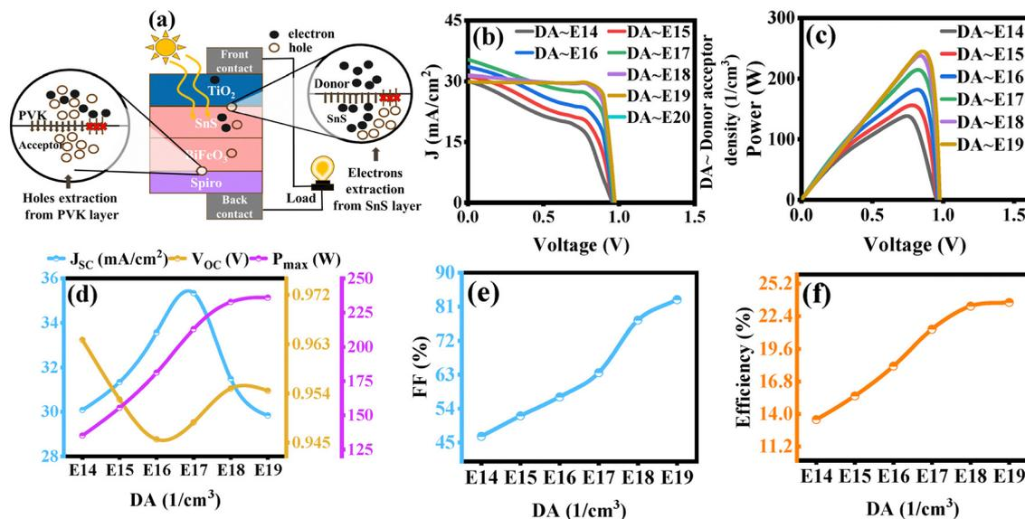
**Fig. 6** (a) Schematic representation of the heterojunction solar cell based on the  $\text{TiO}_2/\text{SnS}/\text{BiFeO}_3$  (PVK)/spiro configuration with carrier transport mechanisms, (b) and (c)  $J$ - $V$  and  $P$ - $V$  response under varying acceptor densities (DA) in the PVK layer, (d) variation in  $J_{sc}$ ,  $V_{oc}$ , and  $P_{max}$ , and (e) and (f) corresponding changes in fill factor and efficiency as a function of DA.
