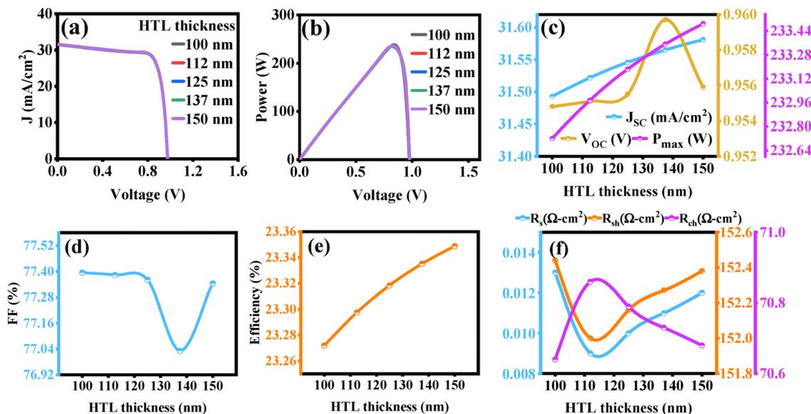
Fig. 5 Effect of HTL thickness variation (100–150 nm) on device ( $\text{TiO}_2/\text{SnS}/\text{BiFeO}_3/\text{spiro}$ ) performance parameters: (a)  $J$ - $V$  characteristics, (b)  $P$ - $V$  response, (c) variation of  $J_{\text{sc}}$ ,  $V_{\text{oc}}$ , and  $P_{\text{max}}$ , (d) and (e) corresponding changes in fill factor and efficiency, and (f)  $R_s$ ,  $R_{\text{sh}}$ , and  $R_{\text{ch}}$  with HTL thickness.
