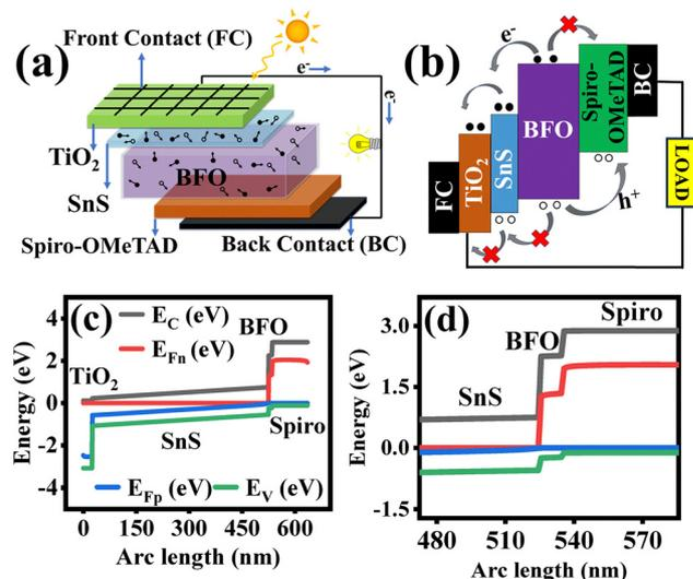
Fig. 2 (a) Schematic representation of the proposed solar cell structure, (b) energy band diagram illustrating the charge transport mechanism under illumination, (c) energy band alignment across the device, indicating conduction band ( $E_{\text{C}}$ ), valence band ( $E_{\text{V}}$ ), and Fermi level ( $E_{\text{F}}$ ) positions, and (d) magnified view of the energy band profile near the BFO/spiro-OMeTAD interface, highlighting carrier extraction dynamics.
