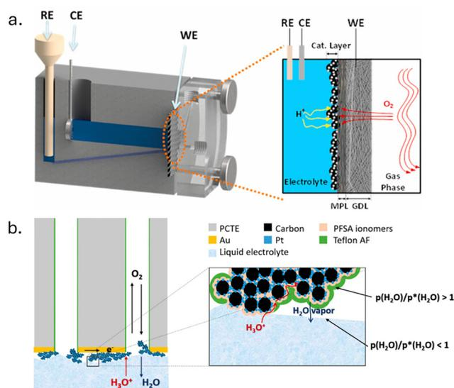
Fig. 8 Schematic configuration of (a) gas diffusion electrode (GDE) half-cell,<sup>86</sup> copyright © 2022 Elsevier B. V., (b) floating electrode (FE) half-cell,<sup>85</sup> copyright © 2020 American Chemical Society.
