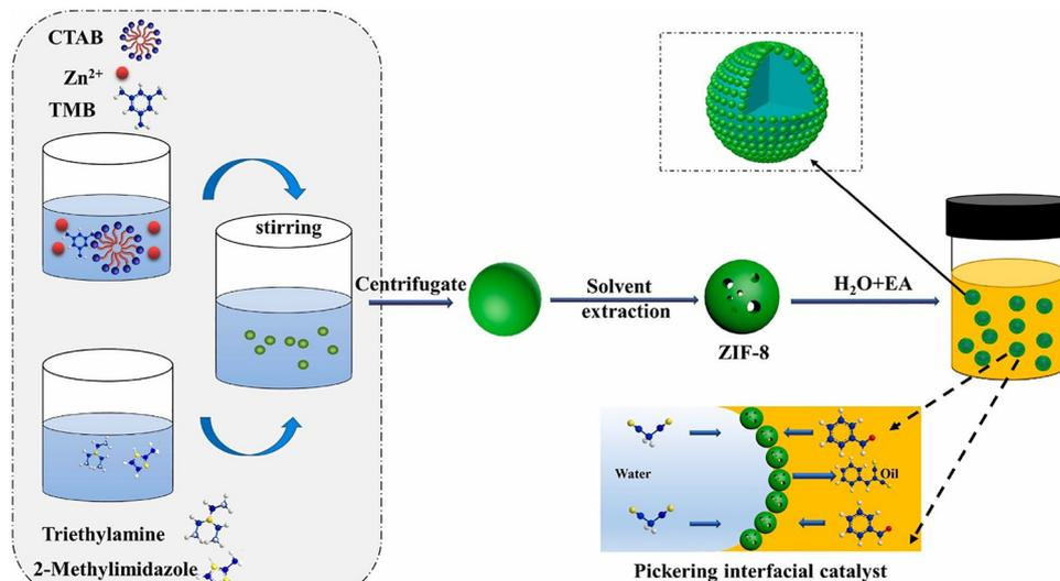
Fig. 7 Schematic of hierarchically porous ZIF-8 formation using TMB-induced pore expansion and Pickering emulsion templating. Reproduce with permission.<sup>72</sup> Copyright © 2021 Elsevier B.V.
