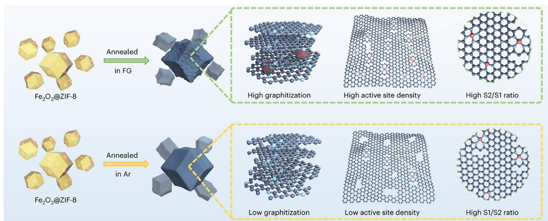
Fig. 1 Schematic of the construction of S1-pyrrolic and S2-pyridinic nitrogen sites through controlled pyrolysis atmosphere. Reproduced with permission.<sup>22</sup> Copyright © 2023 Springer Nature Limited.
