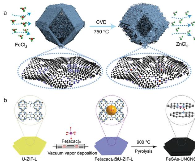
Fig. 4 Schematic CVD synthetic process of Fe–N–C of with (a) FeCl<sub>3</sub>, Reproduce with permission.<sup>50</sup> Copyright © 2021 Springer Nature Limited. (b) Fe(acac)<sub>3</sub>, Reproduce with permission.<sup>51</sup> Copyright © 2024 John Wiley & Sons, Inc or related companies.
