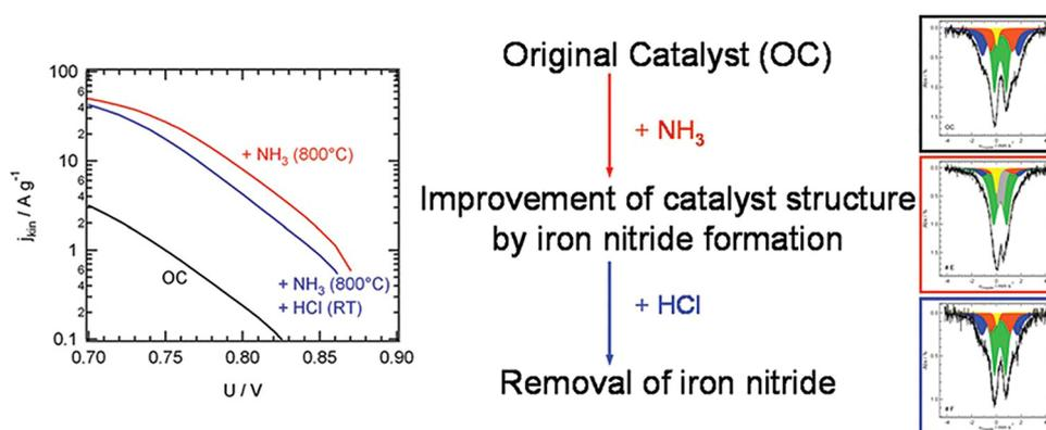
Fig. 2 Fe–N–C structural, Composition and ORR activity evolution of Fe–N–C catalyst upon  $\text{NH}_3$  treatment. Reproduced with permission.<sup>30</sup> Reproduced with permission. Copyright © 2011 American Chemical Society.
