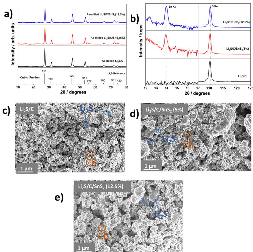
Fig. 2 (a) XRD patterns and (b) XRF spectra of  $\text{Li}_2\text{S}$  composites. SEM images of  $\text{Li}_2\text{S}$  composites (c) without  $\text{SnS}_2$ , (d) with  $\text{SnS}_2$  (5%), and (e) with  $\text{SnS}_2$  (12.5%) additives.
