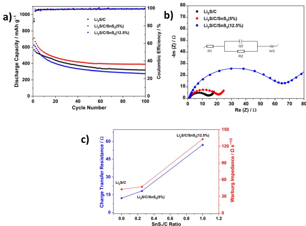
Fig. 4 (a) Cycling performance (including coulombic efficiency) at a current rate of  $C/10$  and (b) Nyquist plots before cycling for  $\text{Li}_2\text{S}/\text{C}$ ,  $\text{Li}_2\text{S}/\text{C}/\text{SnS}_2$  (5%), and  $\text{Li}_2\text{S}/\text{C}/\text{SnS}_2$  (12.5%) electrodes. (c) Linear plot of charge-transfer resistance and Warburg impedance against the  $\text{SnS}_2/\text{C}$  content in the composites.
