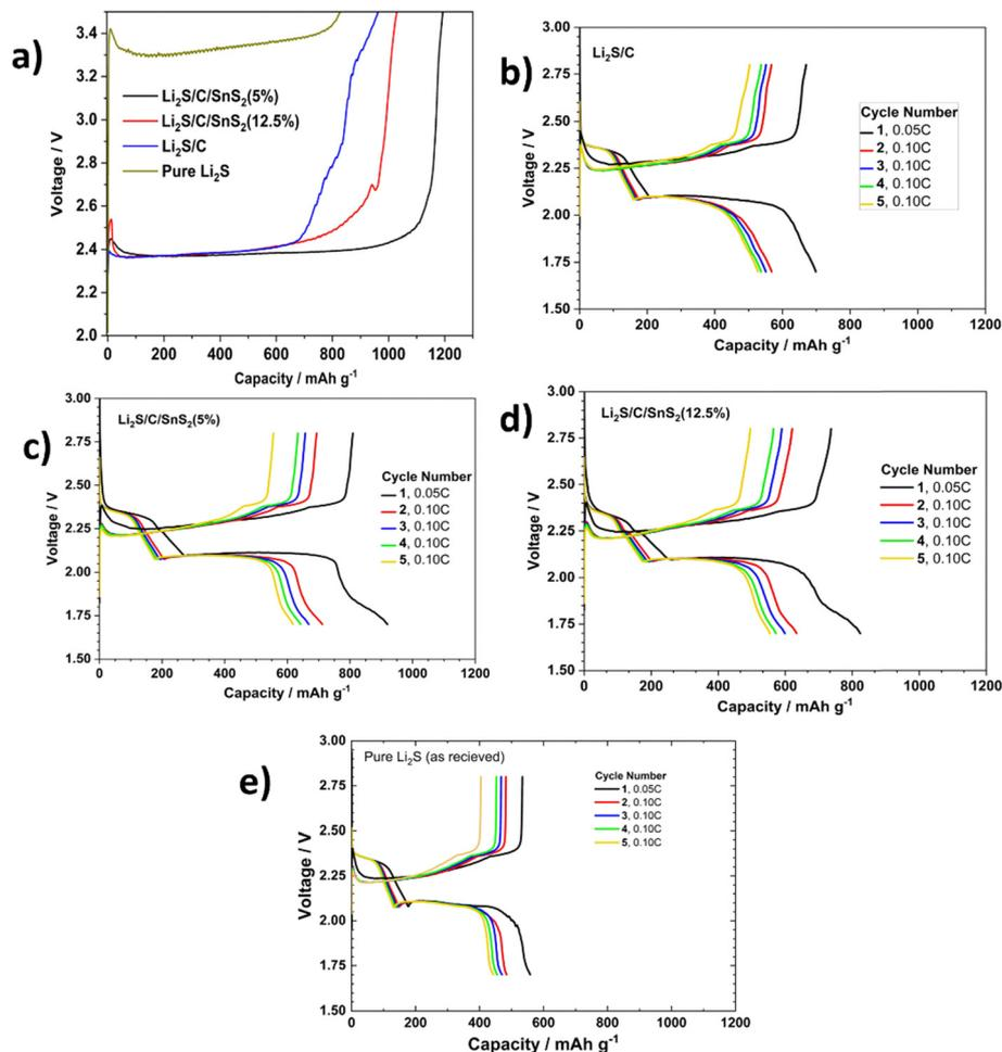
Fig. 3 (a) Charge profiles of the activation process of the as-ball milled  $\text{Li}_2\text{S}$  composites and the as-received  $\text{Li}_2\text{S}$ . The first five galvanostatic charge-discharge curves of  $\text{Li}_2\text{S}$  electrodes after an initial activation: (b)  $\text{Li}_2\text{S}/\text{C}$ , (c)  $\text{Li}_2\text{S}/\text{C}/\text{SnS}_2$  (5%), (d)  $\text{Li}_2\text{S}/\text{C}/\text{SnS}_2$  (12.5%), and (e) pure  $\text{Li}_2\text{S}$ .
