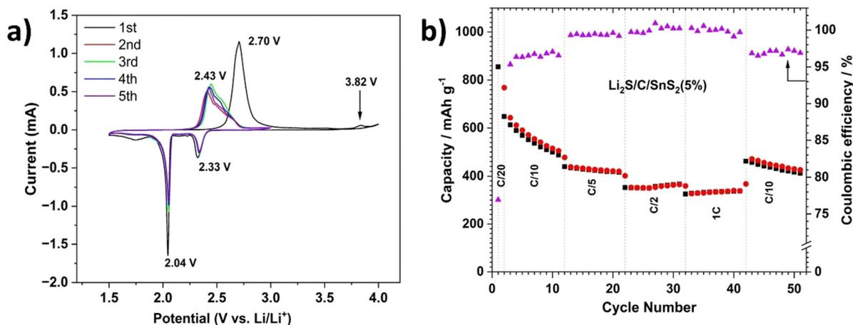
Fig. 5 (a) CV profiles of  $\text{Li}_2\text{S}/\text{C}/\text{SnS}_2$  (5%) electrodes obtained at a scan rate of  $0.1 \text{ mV s}^{-1}$ . (b) Rate performance of  $\text{Li}_2\text{S}/\text{C}/\text{SnS}_2$  (5%) electrodes at a current rate range of C/10 to 1C.
