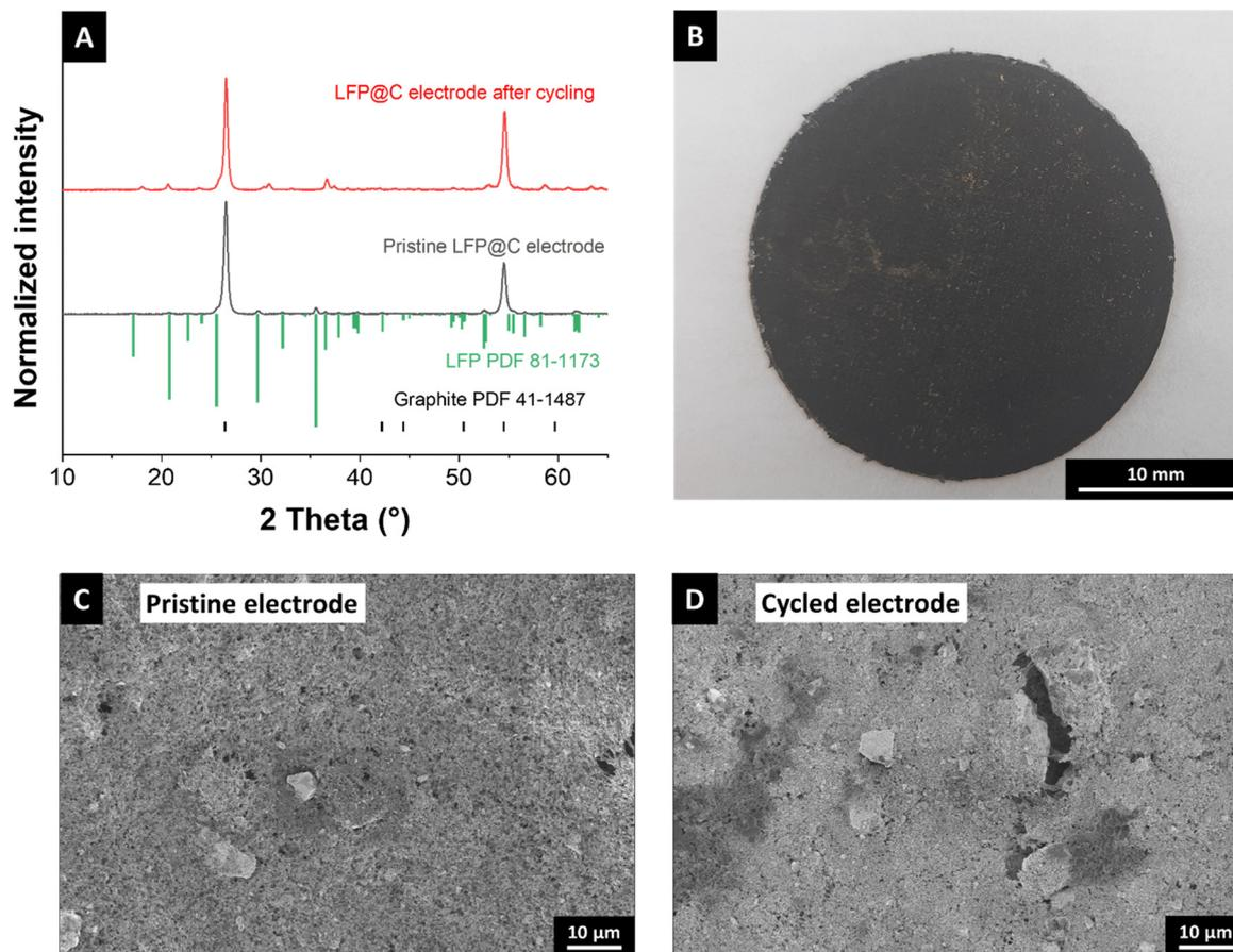
Fig. 7 Post mortem characterization after electrochemical lithium-ion recovery. (A) X-ray diffractograms using Cu-K $\alpha$  radiation for the pristine electrode in comparison to the cycled electrode after 200 cycles. (B) Photograph of the cycled electrode. Scanning electron micrograph of (C) pristine LiFePO $_4$  and (D) cycled (200 cycles) LiFePO $_4$ .
