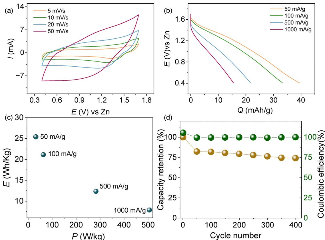
Fig. 5 (a) CV at different sweep rates ranging from  $5 \text{ mV s}^{-1}$  to  $50 \text{ mV s}^{-1}$ , (b) GCD profile at different current rates ( $50 \text{ mA g}^{-1}$  to  $1000 \text{ mA g}^{-1}$ ) of Zn-lignin cells. (c) Ragone plot showing maximum specific energy and maximum power of cell. (d) Capacity retention and coulombic efficiency of the Zn||L/C battery in the WiSH at  $100 \text{ mA g}^{-1}$  of current rate.
