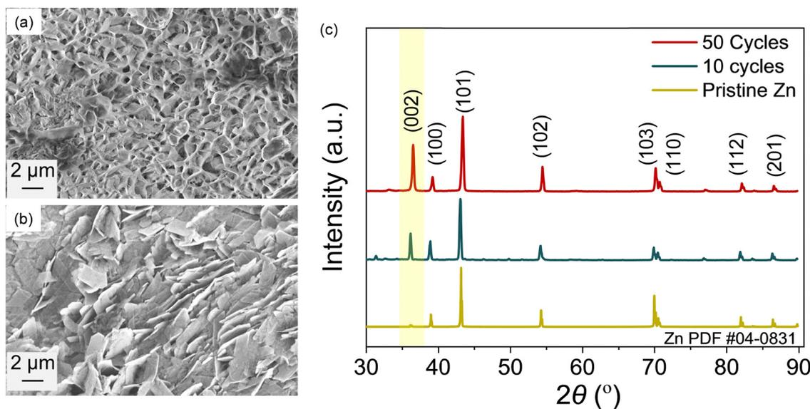
Fig. 2 SEM images of Zn electrodes after galvanostatic plating at 1 mA cm<sup>-2</sup> current rate in 4 m Zn(OTf)<sub>2</sub>-based WiSH: (a) after 10 cycles and (b) after 50 cycles, showing compact and uniform Zn deposition without dendritic structures (scale: 2 μm). (c) XRD patterns of pristine Zn and cycled electrodes after 10 and 50 cycles, revealing a preferential Zn growth along the (002) crystal plane during repeated deposition/stripping in symmetric Zn||Zn cells.
