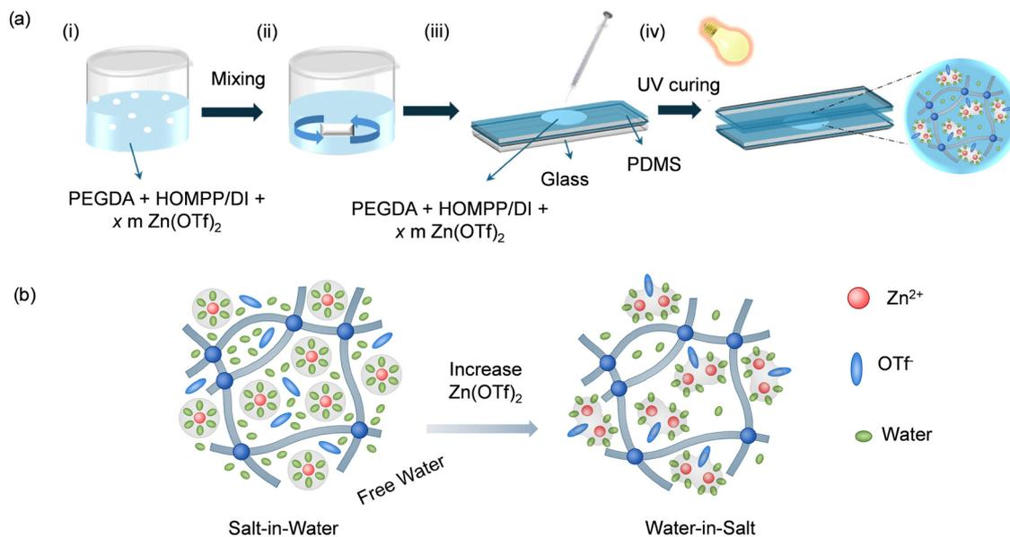
**Scheme 1** Schematic illustration of (a) steps involved to prepare WiSH and (b) the 3-dimensional PEG polymeric network in the hydrogel electrolytes with different  $\text{Zn}(\text{OTf})_2$  ionic salt. Salt-in-water hydrogel electrolyte (left) and WiSH electrolyte (right).
